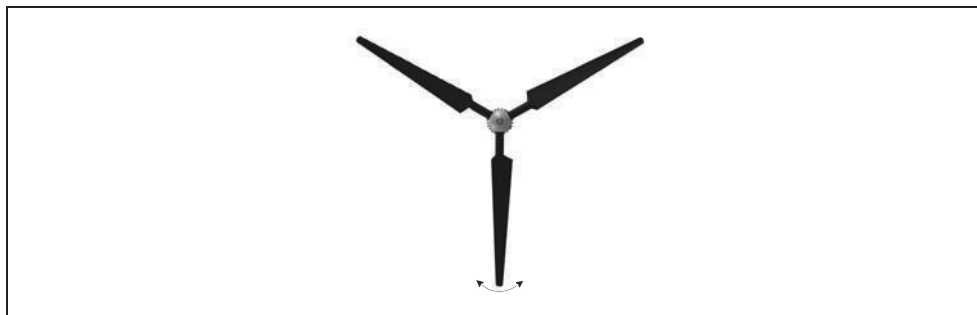
Fig. 7: Balancing the rotor (Y position)
