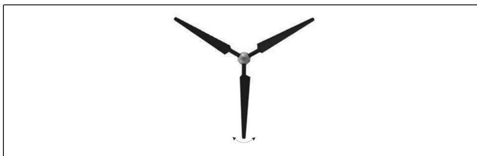
Fig. 7: Balancing the rotor (Y position)
